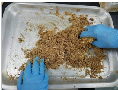
Fig. 1. Mixing of Rice Husk and Adhesive
